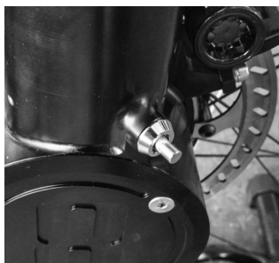
Lock at the bottom of the fork (open, cylinder is out)
