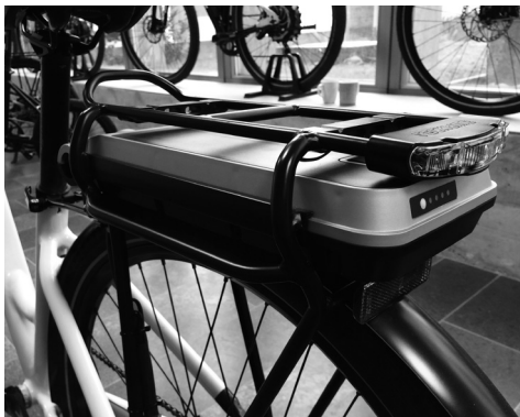
Luggage carrier battery with On/Off button and charge level indicator on the battery
