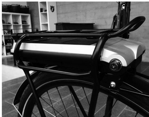
Lock is open, battery can be removed by pressing the unlock mechanism at the rear and pulling
